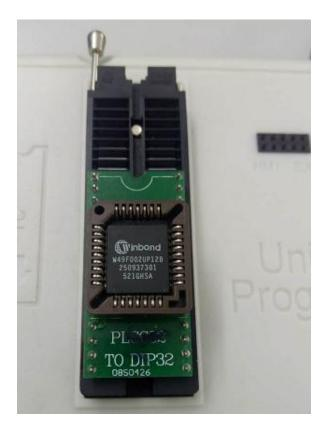
Then input the type in the "Enter chip printing" ,the way of reading, saving and writing are the same with 93XX.
