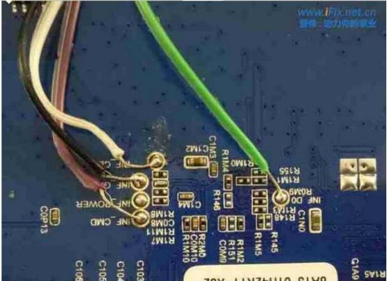
Step 3 : EMMC uses the power supply of board by self,so one line less, just need to supply the 12V power to the board.
