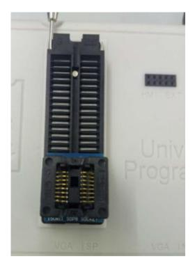
> When using the bounce seat, one foot of the chip should correspond to the top left corner.
