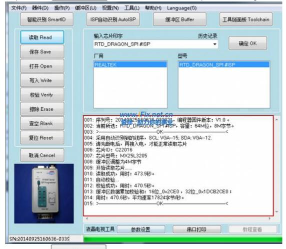
Step 4 : Click to save the file after finishing reading. Try the best to name the file in detail, including the manufacturer, board number, screen type, main chip type, memorizer type for the convenient use in the later.
