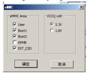
Step 2: If the EMMC\_AUTO\_8BIT can't work,use the EMMC\_AUTO\_4BIT to have a try; If it can't work by reading four areas on the left,try to read a area alone; Exchange the chip of same type to try(make sure of the chip well or not); Fly line reading EMMC mistake:
